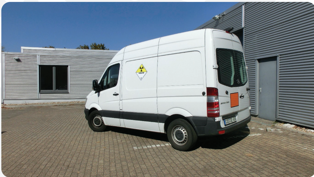
Vehicle signage with orange warning sign and class 7 transport sign
