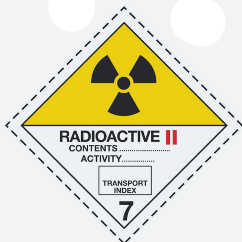
Example: Hazard labels for radioactive substances
