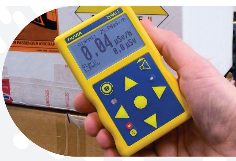
NUVIATech Instruments presents the new powerful DolMo product line. In combination with our useroriented accessories, the DolMo product line is the new solution for dose, dose rate and contamination measurements. The compact measurement devices are the ideal instruments for your daily work operations.
