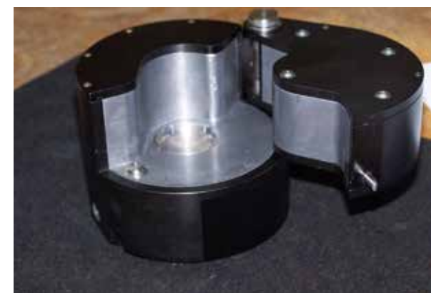
Shielding container designed for easy transport of irradiated target and optional loading into the CRAB
