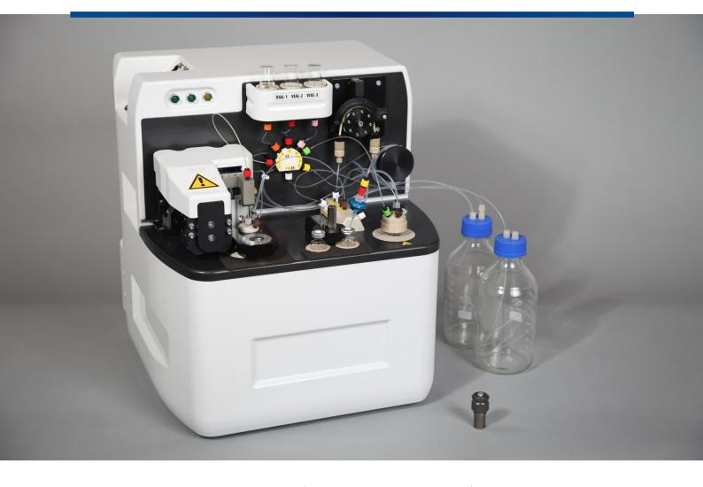
OCTOPUS is a system designed for automated processing of neutron-irradiated, <sup>176</sup>Lu enriched targets. The process involves dissolution of the target, evaporation to dryness and re-dissolution of the residue in an appropriate solvent in order to obtain <sup>177</sup>Lu solution intended for radiolabelling. The device is also capable of dispensing the product.
