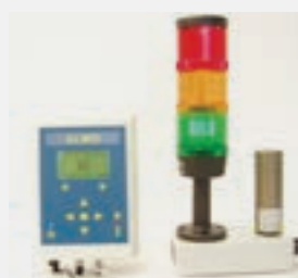
Area monitoring system NuRMS ALMO Dose rate monitoring system available in special clean room versions or to be integrated into networks for central measuring value display and alarm indications
