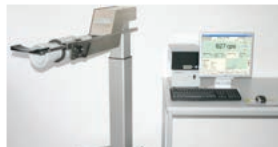
Thyroid uptake counter NuMED ISOMED 2162 designed to determine activity of ^{131}\text{I} in thyroids in the radiotherapy ward
