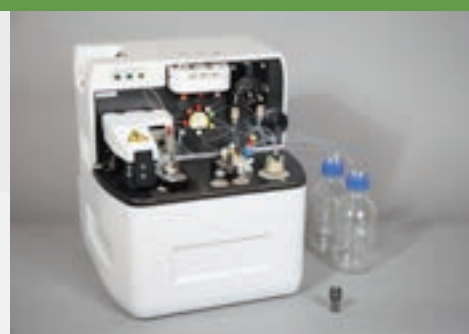
NuARP OCTOPUS Device for processing ^{176}\text{Lu} -enriched oxide targets to prepare ^{177}\text{Lu} radionuclide precursor for radiolabelling
