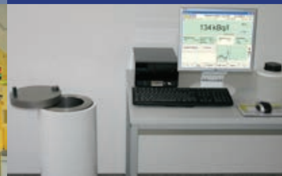
Waste water counter NuWM ISOMED 2151 For the measurement of the activity of radionuclides contained in the waste water produced in nuclear-medical facilities and radioiodine wards.
